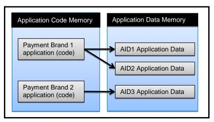
Figure 1: Example of Multi-Application EMV Card Structure
